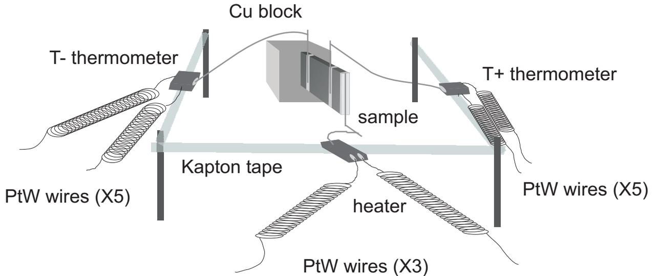
Figure 4.2: A Schematic diagram of a mount used in our measurements of thermal conductivity. The geometry is dubbed “the washing line configuration” since the thermometers and heater are suspended by  $7\mu\text{m}$  thick Kapton tape strung up between Vespel posts. Heat is provided by passing current through a resistive strain gauge, and temperature is recorded by measuring the resistance of  $\text{RuO}_2$  chips.
