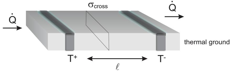
Figure 4.1: Schematic diagram depicting the one heater two thermometer method of thermal conductivity measurement. The heat flows in through one face of the crystal to thermal ground, and the resulting thermal gradient is measure at two thermometers denoted by  $T^+$  and  $T^-$ .
