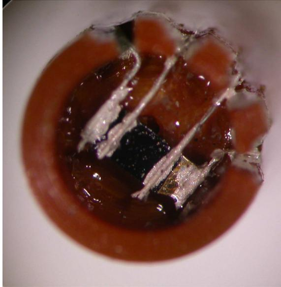
Figure 4.5: Resistivity mount for measurements in pulsed magnetic fields. The probe inserted such that the magnetic field is  $\perp$  to the face of the crystal.
