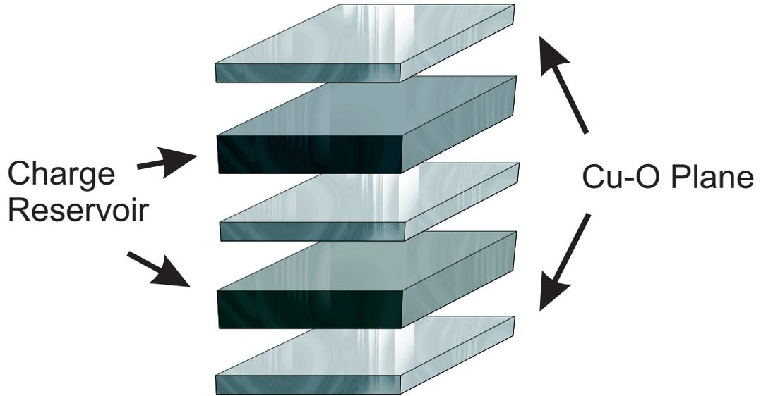
Figure 1.1: The basic building blocks of a cuprate superconductor. Cu-O planes host electronic transport, separated by charge reservoir layers which either serve to dope holes or electrons into the planes.
